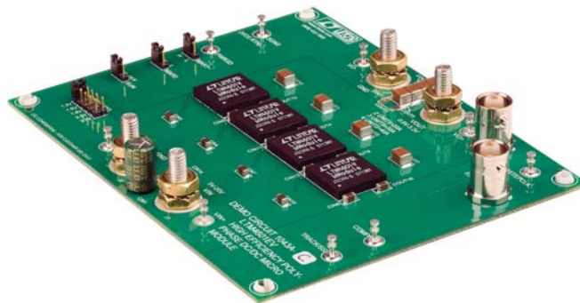
Figure 1. Four DC/DC \mu Module Regulator Systems Current Share to Regulate 1.5V at 48A With Only 2.8mm Profile and 15mm \times 15mm of Board Area for Each Device. Each \mu Module Regulator Weighs Only 1.7g and Has an IC Form-Factor that Can Easily be Used With Any Pick-and-Place Machine During Board Assembly
